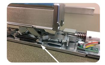
**9.** SLIDE THE HOUSING BACK ONTO THE BASERAIL MAKING SURE THE MOTOR & BASERAIL ARE IN THE CORRECT CHANNEL. BE CAUTIONS OF PINCHING MOTOR/REX WIRES.
