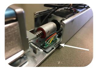
**10.** RE-INSTALL (2) SCREWS ON MOUNTING BRACKET WITH 5/16" NUT DRIVER.
