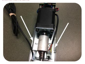
**8.** VISUALLY CONFIRM HOOKS ARE ATTACHED TO ROLL PIN. IF NOT REPEAT STEP B.
